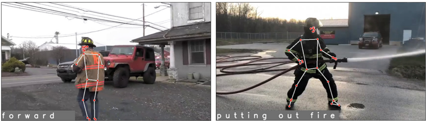
Fig. 3. The automated annotation on videos. Left = Moving forward, Right = Putting out fire
